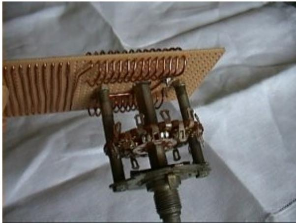
These pictures show the actual construction of coils A; B; and C after having been mounted on the switch assembly, but prior to wiring.
