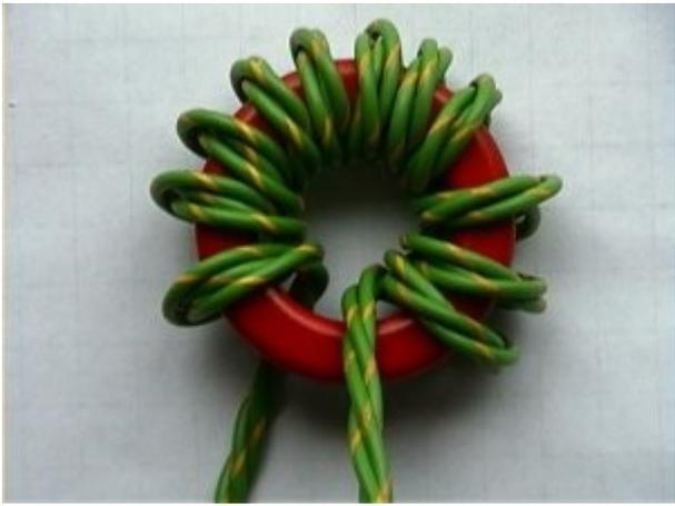
Construction of coils A; B; C; and D
